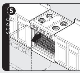
If leveling is required, move unit out of opening.
