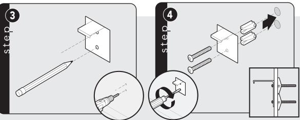
Mark and drill holes where bracket will be located
