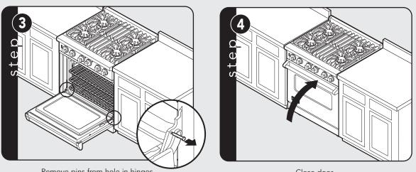
Remove pins from hole in hinges.
