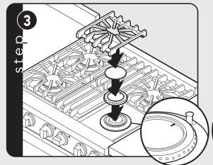
Burner caps are packed in styrofoam top pack with the grates. Place burner on top of range. Place burner grate on top of burner cap and grate support. **Note:** Arrow on burner cap must be pointing towards back of range.
