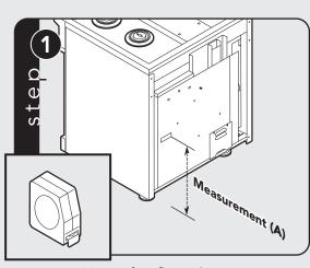
Locate anti-tip bracket on rear wall with the top left corner at measurement (A) plus 1/2" (1.3 cm) from the floor and 3-5/8" (9.2 cm) from where the right side of range (facing range) is to be located.
