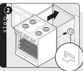
Slide range into place. Be sure anit-tip bracket slides into the anit-tip opening.
