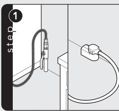
Connect gas and electrical. Before placing appliance in operation, always check for gas leaks. This must be performed by your dealer, a qualified licensed plumber, or gas service company.
