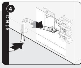
Feed supply cord up through hole in bottom of range back.
