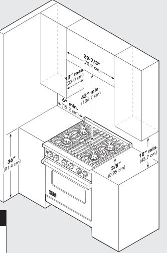
Note: Minimum clearance for back wall is 0" with backguard or high-shelf.
