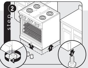
Note: It is strongly recommended that a pallet or lift jack be used rather than tilting. Raise unit about a foot. Unscrew temporary legs from couplings on all four corners.
