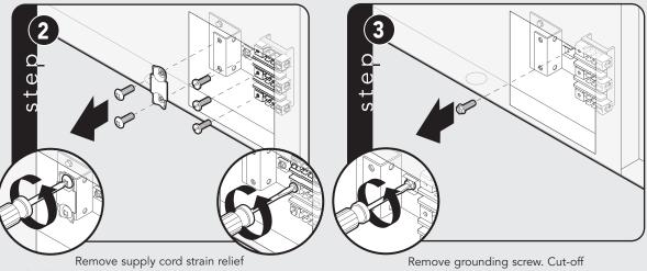
bracket and three supply cord mounting screws on the terminal block.
