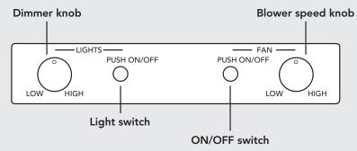
**ON/OFF switch**—Starts and stops the blower. When turned on the blower will operate at the previous setting of the speed control.
