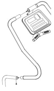
**STEP 8 CONSOLE** • Remove the four screws from the back of the console. Plug the wire connectors from inside the mast into the console. The cable connectors are slotted, so do not force the
