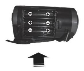
Insert 3 x AA batteries as shown above.
