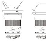
The hood has a bayonet system, which guarantees speedy, efficient, safe and precise installation and will help you take shots that are free of flaring and ghosting. Allign the attachment reference point on the hood with the reference point on the lens. Push the hood onto the lens and turn the hood to the right until it makes a clicking sound.
