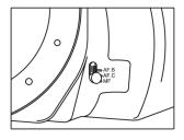
3. Set the focus adjustment lever of the camera to "MF".
