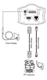
Shut down all the peripheral devices prior to connection. Connect the supplied cables from Network Camera to related devices according to the following steps. Note that the power adaptor must be kept unplugged until other cables are firmly connected.
