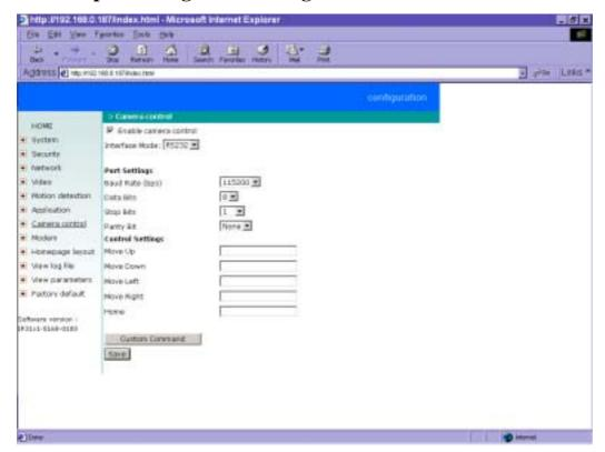
Since Network Camera can be used in either PPP network or Ethernet network, the single serial port can control either external serial port devices like camera positioning devices or a data modem. While in PPP interface, go to Modem page for modem configuration. Options on this page will be ignored.
