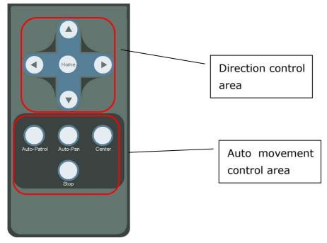
"**Auto Patrol**" This button commands the camera to patrol between the preset positions on the patrol list that was set on the "Camera control page". After each patrol cycle, the camera stops at the original staring position. "**Auto Pan**" This button commands the camera to pan from the current position to the left most or right most and back. After panning both horizontal end positions, the camera would stop at the original starting position.
