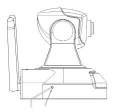
Restoring the factory defaults will erase any previous settings. Reset or restore the system after power on. At the left side of the camera there is a button hidden in the pinhole as shown in the picture. It is used to reset the system or restore the factory default settings. Sometimes resetting the system sets the system back to normal state. If the system problems remain after reset, restore the factory settings and install again.
