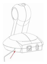
There is a button in the back side of the Network Camera. It is used to reset the system or restore the factory default settings.
