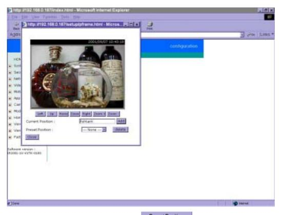
To preset the camera head position, press Preset Position and another window will pop up with the camera view and control buttons for preview. After moving it to the desired position, enter the preset position name and click on Add. Note that if improper characters are used in the position name, a warning message window will pop up.
