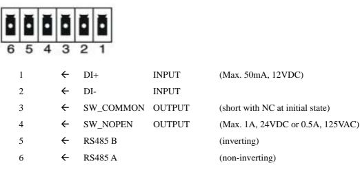
VisualServer provides a very flexible general I/O interface to combine with the user's security devices such as sensors, alarms, lighting or door locks. The general I/O terminal block has six pins for device control. These pins can be divided into two categories based on their functions, including RS485 and digital inputs and outputs.
