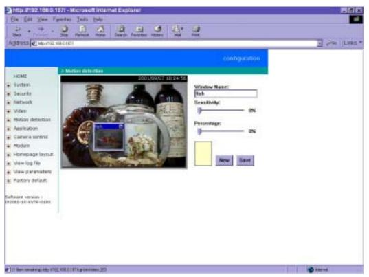
Please note that the option "Enable Motion Detection" on the video page must be enabled to make detection effective.
