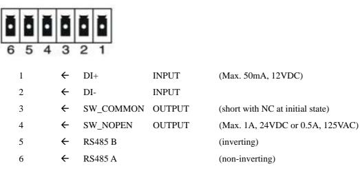
NetworKam provides a very flexible general I/O interface to combine with the user's security devices such as sensors, alarms, lighting or door locks. The general I/O terminal block has six pins for device control. These pins can be divided into two categories based on their functions, including RS485 and digital inputs and outputs.
