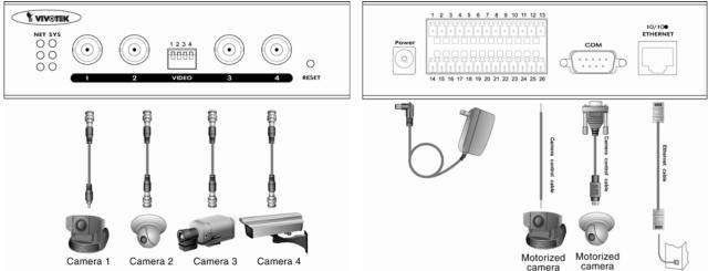
Shut down all the peripheral devices prior to connection. The video BNC, Ethernet cable and power adapter are essential for basic viewing function. If the attached cameras belong to the same motorized model, they can be concatenated to single COM port and will be differed by camera ID set on the cameras. Refer to the related configuration section for detailed description.
