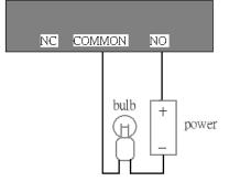
If DI1 in configuration is set as rising to drive DO1 to high that denotes COMMON of DO1 short with NO, then the bulb will light when DI1 signal changes from 0V to 12V.
