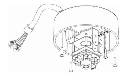
2. Fix the camera to the wall/ceiling with four supplied screws
