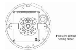
Restoring the factory defaults will erase any previous settings. Reset or restore the system after power on.
