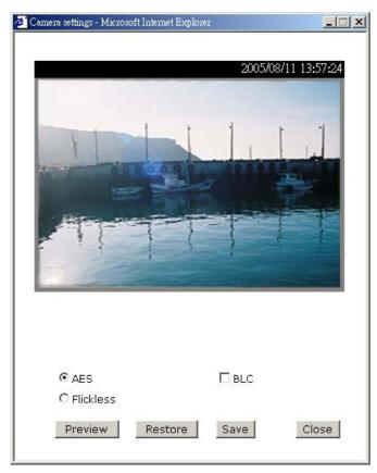
**"AES" -** auto electronic shutter, enable this will let CCD sensor adjust electronic shutter automatically.
