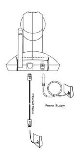
Please verify that your product package contains all the accessories listed in the foregoing Package Contents. Depending on the user's application, an Ethernet cable may be needed. The Ethernet cable should meet the specs of UTP Category 5 and not exceed 100 meters in length.
