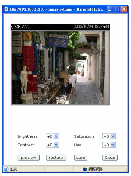
"Contrast", "Hue" and "Saturation" for video compensation. Each field has eleven levels ranged from -5 to +5. In "Brightness" and "Contrast" fields the value 0 indicates auto tuning. The user Preview press to fine-tune the image. When the image is O.K., press save to set the image settings. Restore Click on this to recall the original settings without incorporating the changes.
