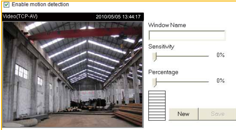
Motion Detection Setting 1: For normal situations
