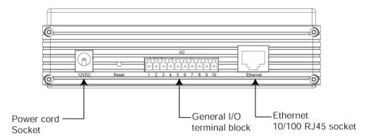
"Power cord socket" Plug the power jack of the included power adapter to Video Receiver. Connecting the power adapter should be the last operation while physically installing Video Receiver.
