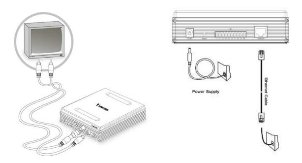
Please verify that your product package contains all the accessories listed in the foregoing Package Contents. Depending on the user's application, an Ethernet cable may be needed. The Ethernet cable should meet the specs of UTP Category 5 and not exceed 100 meters in length.
