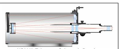
VC200L Telescope Schematic Drawing
