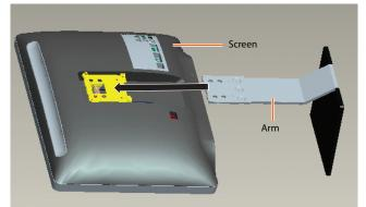
4 Insert the thumbscrew into the mounting hole on the back of the arm, then tighten the thumbscrew to secure your monitor to the arm.
