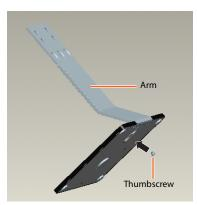
**3** Lay your monitor screen face-down on a padded surface, such as a towel, then slide the arm into the mounting bracket on the back of the screen.
