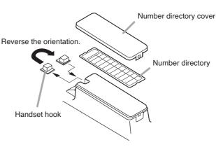
**Step 3.** After replacing the directory on the station, hook the directory cover's forward tab and push on the upper part of the directory cover.
