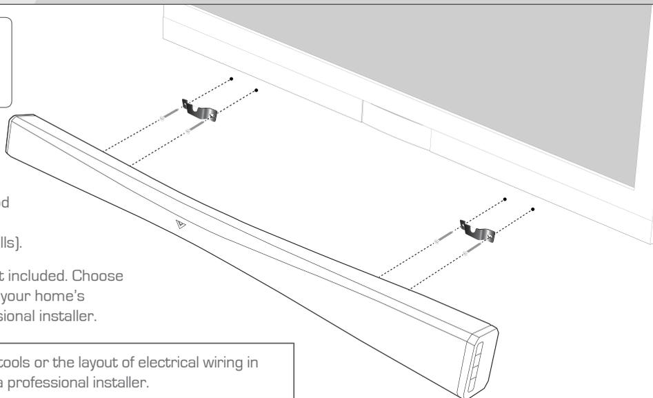
Be sure your screws are attached to wood studs or drywall anchors (for drywall) or concrete anchors (for brick/concrete walls).
