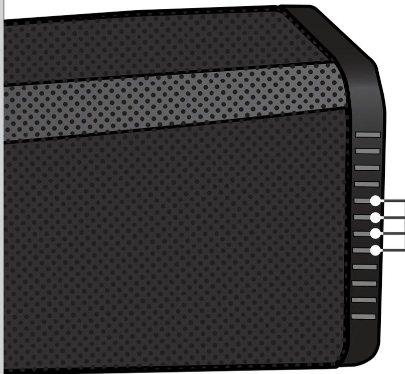
When the four center Indicator LEDs are brightly lit, the selected SRS mode is enabled. When the LEDs are not lit, SRS mode is disabled.
