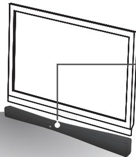
When using the remote, point it at the center of the Sound Bar. The sensor is located there.
