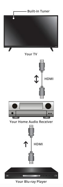
HDMI ARC transmits all-digital audio from your TV to your home audio receiver, with no need for an extra cable. The single HDMI cable also carries digital HD (high definition) video to your TV.
