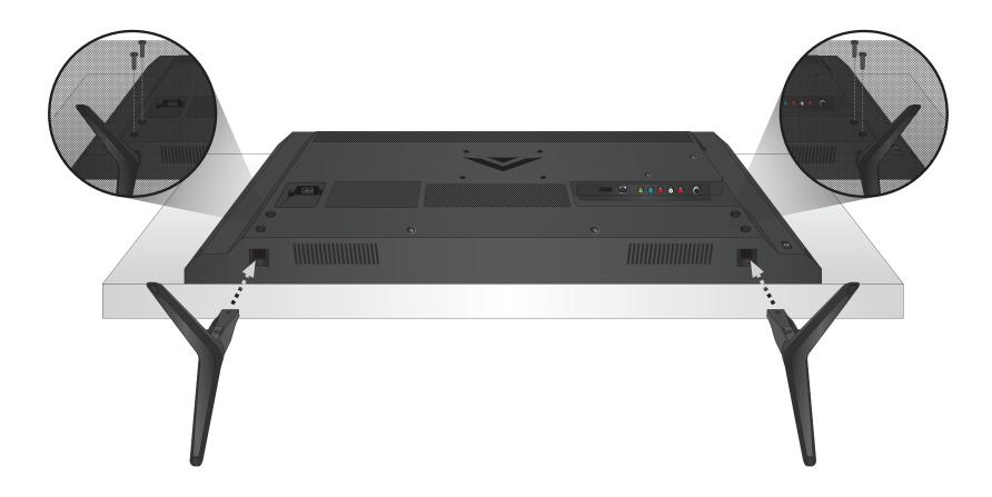
Insert the left and right stands into the base of the TV (the stands are identical).
