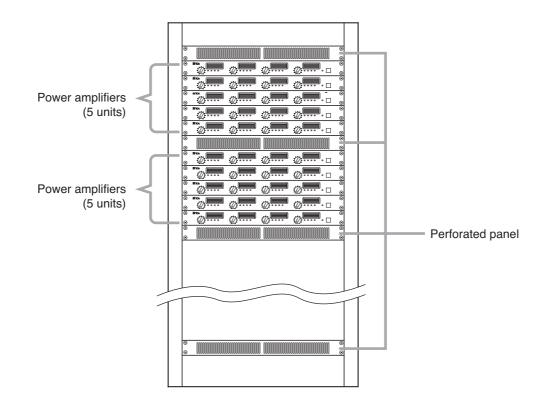
• Robust structure is one of the unit's main features. However, if the strength is particularly needed when installing the unit in the rack, use a supporting runner for the safety purposes.
