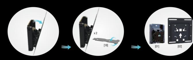
Remove the screen plate by removing the two screws and saving one for later to tighten the screen plate to the wall plate.
