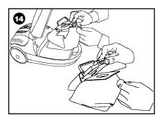
Your appliance is equipped with a dust bag. If you notice that the vacuum cleaner seems to be less efficient than usual, check the dust indicator by selecting the maximum power and lifting the cleaner tool off the floor. If the indicator turns red, change the bag.
