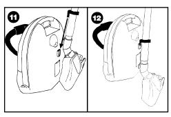
Fig.10 If you wish to pause briefly during vacuuming i.e. to move a piece of furniture or a rug, use the special parking position on your vacuum cleaner. Slide the hook attached to the large cleaning tool into the slot on the rear of the appliance. When you have finished vacuuming, press pedal to stop the appliance then unplug it at the mains. Press the pedal to automatically rewind the cord (See note fig.6).
