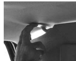
6. With the visor now in service position, pull the visor bracket down. This will remove the visor completely from the roof header and headliner.
