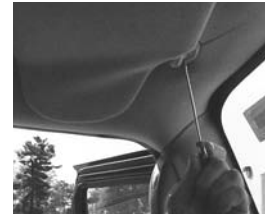
1. Use a small blade screwdriver to insert in access slot to depress the retaining tab.
