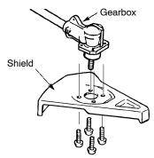
Insert the 4 mounting screws through the bottom of the shield. Thread them into the gearbox. Tighten evenly and securely with one of the hex key wrenches provided.
