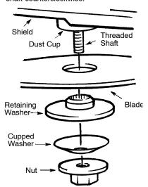
**WARNING:** Do not use any blades, or fastening hardware other than the washers and nuts illustrated. These parts must be provided by Weed Eater, and installed as shown below. Failure to use proper parts can cause the blade to fly off and seriously hurt you or others
