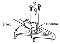
Insert and thread the 4 mounting screws through the holes of the gearbox and the metal shield. Tighten evenly and securely with the hex wrench provided.
