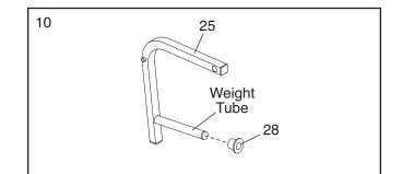
Attach a Fly Arm (25) to an Upright (1) with an M10 x 120mm Bolt (19) and an M10 Locknut (33). Make sure that the Fly Arm is resting against the outer side of the Fly Arm Stop (15). Do not overtighten the Locknut; the Fly Arm must pivot easily.
