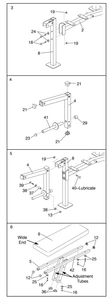
Lubricate the M10 x 178mm Bolt (17). Attach the Backrest (6) to the Frame (2) with the Bolt, two M10 Washers (24), and an M10 Nylon Locknut (19).
