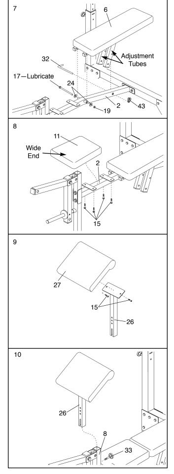
Slide the Curl Post (26) into the Front Leg (8). Align one of the adjustment holes in the Curl Post with the adjustment hole in the Front Leg. Tighten the M10 x 48mm Adjustment Knob (33) into the adjustment hole in the Front Leg. Make sure that you fully tighten the Adjustment Knob.
