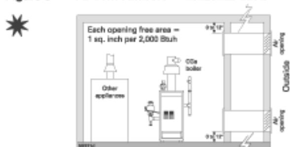
Figure 5 Air from outdoors – horizontal ducts
