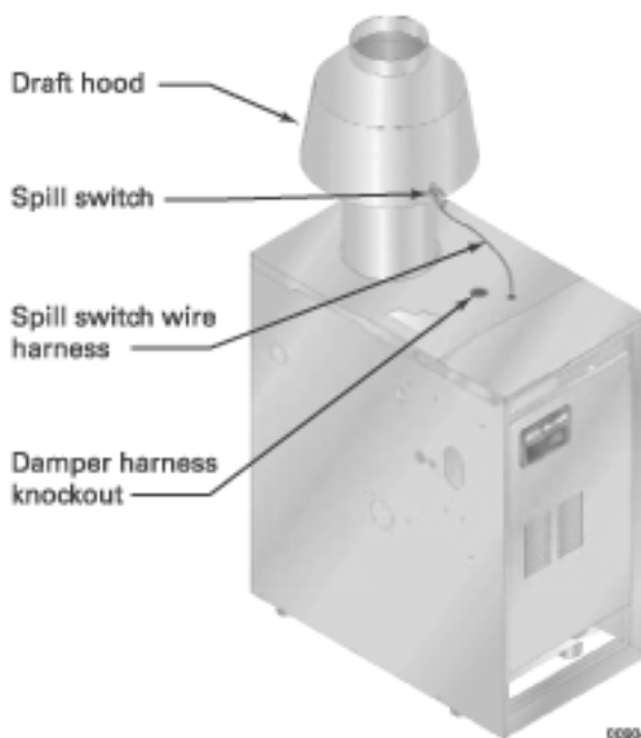
Figure 7 Spill switch with wire harness
