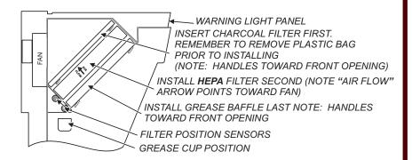
Remove the protective plastic bag from charcoal filter before installing.
