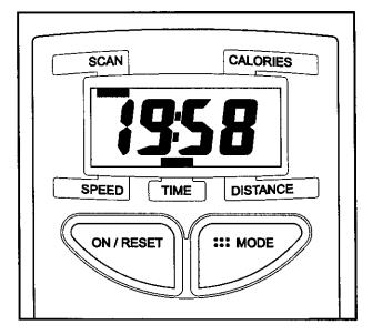
Speed—This mode displays your pedaling speed, in miles per hour or kilometers per hour.
