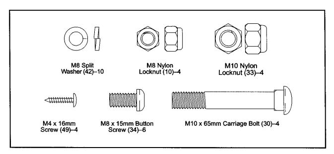
1. While another person lifts the front of the Frame (1) slightly, attach a Stabilizer (2) with two M10 x 65mm Carriage Bolts (30) and two M10 Nylon Locknuts (33).
