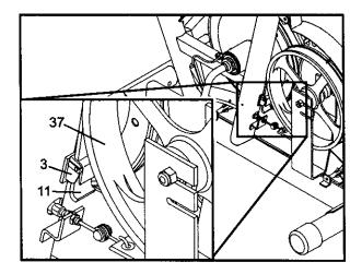
When the resistance strap is properly adjusted, reattach the left side shield and the left pedal.
