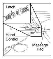
3. Fold the massage chair into the storage position. Slide the massage pad off the seat frame and the back frame. Note: There is a sleeve between the massage pad and the frame. Be careful not to remove the sleeve as you remove the massage pad.
