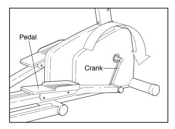
To dismount the ECLIPSE, allow the pedals to slowly come to a stop. **CAUTION:** The ECLIPSE does not have a freewheel; the pedals will continue to move until the flywheel stops. When the pedals are stationary, step off the highest pedal first. Then, step off the lowest pedal.
