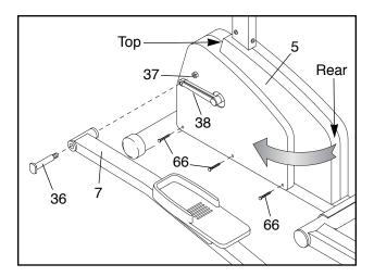
Remove the three M4 x 38mm Screws (66) from the bottom of the Left Side Shield (5). Grasp both Side Shields at the top and gently pull them apart. Make sure that the arm of the Crank (38) is in the position shown in the drawing above. Hold the Left Side Shield at the rear and pull it gently away from the frame. Work the Left Side Shield forward off the arm of the Crank and remove it.
