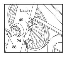
pull it down to remove any slack. While holding the end of the Tension Belt, close the latch on the Tension Belt Clamp. Turn the Crank (38) for a moment to make sure that there is not too much resistance. When the resistance strap is properly adjusted, reattach the left side shield.
