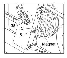
Screw. Turn the Crank (38) for a moment. Repeat until the console displays correct feedback. When the Reed Switch is correctly adjusted, reattach the left side shield.
