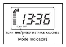
a second mode indicator will show which mode is currently displayed. Note: If a different mode is selected, you can select the scan mode again by repeatedly pressing the mode button. Time, speed, distance, or calories mode—To select one of these modes for continuous display, press the mode button
