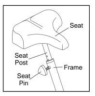
pin counterclockwise to remove it. Next, align a different hole in the seat post with the hole in the frame, and insert the seat pin into the frame and the seat post. **Make sure to insert the seat pin into the seat post; do not insert the seat pin under the seat post.** Tighten the seat pin into the frame.
