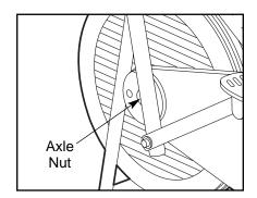
straight and retighten the axle nuts.
