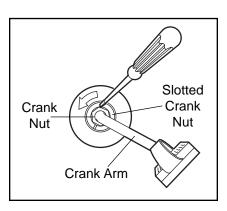
Place the end of a standard screwdriver in one of the slots in the slotted crank nut. Lightly tap the screwdriver with a hammer to turn the slotted crank nut counterclockwise until the arms are no longer loose. **Do not overtighten the slotted crank nut.** When the slotted crank nut is properly tightened, retighten the crank nut.
