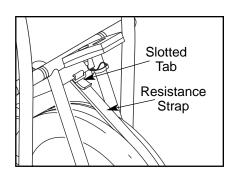
longest part the resistance strap underneath the slotted tab and pull it towards the slot. When a little slack is created, pull the end of the resistance strap tight. Turn the crank for a moment to make sure that there is not too much resistance.
