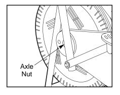
straight and retighten the axle nuts.
