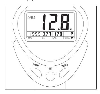
**Speed**—This display shows your pedaling speed, in miles or kilometers per hour.
