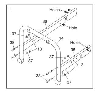
2. Raise the Left Upright (35) and the Right Upright (36) to the position shown. Feed the Reed Switch Wire (6) into the top of the Left Upright and out of the indicated hole.
