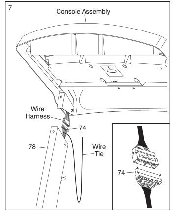
8. Insert the wires into the Right Upright (78). Next, insert the brackets on the console assembly into the Right Upright and the Left Upright (77). **Be careful not to pinch any wires.**
