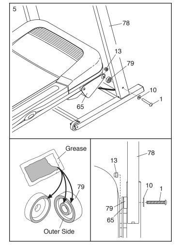
6. **See the left inset drawing.** Identify the outer side of the remaining Frame Spacer (79).
