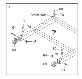
2. Raise the Base (79) to a vertical position, and hold it near the treadmill Frame (96) as shown. Make sure that the Wheels (63) are in the indicated position.
