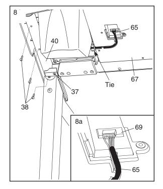
9. Press the Wire Harness (65) into the indicated track in the Console Base (67). (Note: If there is a cylinder on the Wire Harness that will not fit into the track, press as much of the Wire Harness as possible into the track.) Next, insert the excess Wire Harness into the large hole in the side of the Right Handrail (40). Securely tighten the nylon tie to prevent the Wire Harness from slipping, and then cut off the end of the nylon tie.
