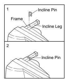
treadmill on its right side. Repeat the procedure for the left incline leg.
