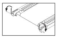
adjustment bolt clockwise, 1/4 of a turn each. Be careful not to overtighten the walking belt. Walk on the treadmill for a few minutes. Repeat until the walking belt is centred.
