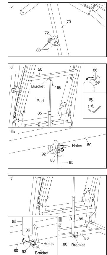
Identify the rod end of the Gas Spring (85). See the two small inset drawings. Locate the Spring Clip (86) in the rod end of the Gas Spring. Using your fingernail or a screwdriver, press on the end of the Spring Clip to loosen it. Rotate the Spring Clip, and then pull the Spring Clip out of the Gas Spring. Avoid losing the Spring Clip. Extra Spring Clips are included.
