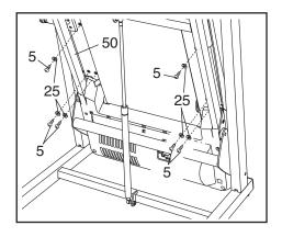
Remove the five indicated M4.2 x 19mm Washer Head Screws (9). Then, carefully remove the Motor Hood (56).
