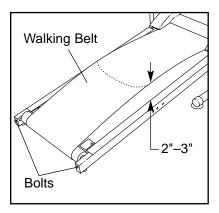
wrench, turn both rear roller adjustment bolts counterclockwise 1/4 of a turn. When the tension of the walking belt is correct, you should be able to lift each side of the walking belt 2 to 3 inches. Walk on the treadmill for a few minutes. Repeat until the walking belt is properly tightened. Be careful to keep the walking belt centered.
