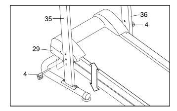
**A** CAUTION: Make sure both Pins (4) are fully inserted at the same height.
