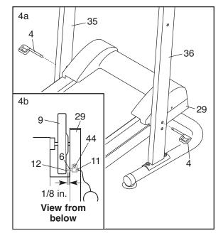
Hold the Handrail (5) near the Left and Right Uprights (35, 36). Connect the Handrail Wire (2) to the Reed Switch Wire (6). Insert the Wires down into the Left Upright.
