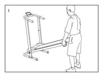
2. Hold the treadmill securely with your left hand as shown. Insert the Storage Pin (42) into the hole in the right side of the Right Upright (36) and into the Frame (29) as far as it will go.
