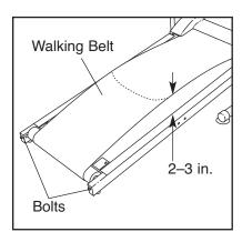
hex key, turn both rear roller adjustment bolts counterclockwise 1/4 of a turn. When the walking belt is properly tightened, you should be able to lift each edge of the walking belt 2 to 3 in. (5 to 7 cm) off the walking platform. Be careful to keep the walking belt centered. Walk on the treadmill for a few minutes. Repeat until the walking belt is properly tightened.
