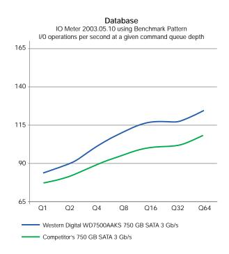
After extensive drive testing, *Tom's Hardware* proclaims, "With peak data rates up to 95 MB/s, the 750 GB top-of-the-line member in the Caviar SE16 family is the fastest 7,200 RPM hard disk we've seen in our test labs to date." The review continues, "...our benchmarks should give WD plenty to cheer about. In particular, the I/O performance in the file server and database server schemas is noticeably superior to that of other 7,200 RPM drives." (As evidenced by the graphs above.)
