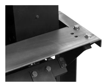
A. Using Drilling Plan "A", drill and counter sink two .375" holes in both the left and right Breaker side plates.
