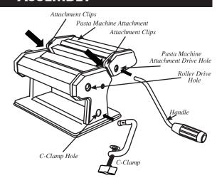
5. Slide the **Handle** into the **Drive Hole** of the **Roller** or the **Attachment** to be used. Be sure to notice when the **Handle** turns, it passes below the edge of the work surface and turns freely.
