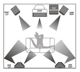
System using conventional rear speakers
