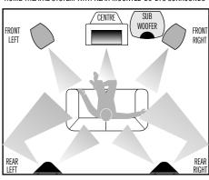
Many digital AV Processors require you to specify the size of speakers in the various channels. These are usually 'Large' or 'Small'. The Rear and Centre channels should be set to 'Small'.
